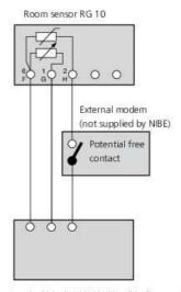
Connection to be done on terminal block 14/X1/X4 in all before mentioned heat pumps and electric boilers. Note that connection to ACVM 270 must be carried out according to section "Connecting external contacts" in the product's Installation and Maintenance instructions.
