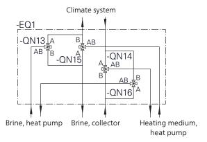
Install the three-way valves according to the outline diagram above.
