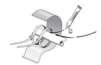
Install the temperature sensors using cable ties, together with the heat conducting paste and aluminium tape. Then insulate with the enclosed insulation tape.
