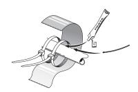
Install the temperature sensors with cable ties with the heat conducting paste and aluminium tape. Then insulate with supplied insulation tape.
