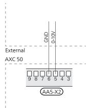
0V is 0% of the minimum speed of the pump and 10V is 100% of the maximum speed of the pump.
