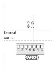
At 0 V the shunt is closed and at 10 V the shunt is open.
