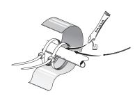
Install the temperature sensors using cable ties, together with the heat conducting paste and aluminium tape. Then insulate with the enclosed insulation tape.
