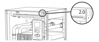
This accessory contains an accessory board (AA5) that must be connected directly to the heat pump on terminal block X6 in F1345 or on terminal block AA101-X10 in F1345 2.0/F1355.
