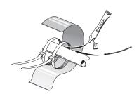
Install the temperature sensors using cable ties, together with the heat conducting paste and aluminium tape. Then insulate with the enclosed insulation tape.
